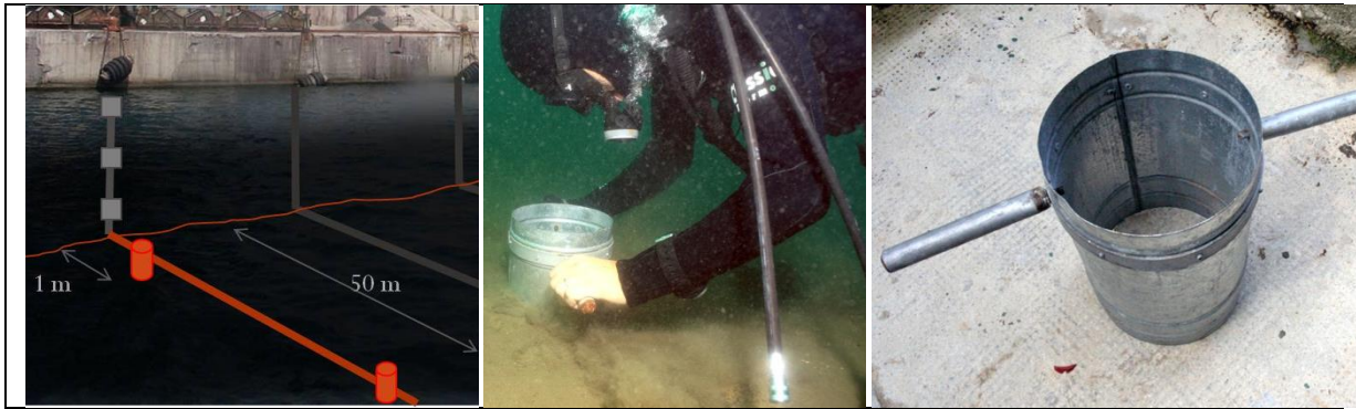
Figure 5- Infauna sampling on 50 m long transect using hand corer ( \varnothing = 18 cm, h = 30 cm).
