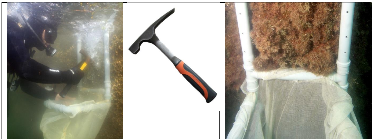
Figure 4- Sampling on sampling plot using brick hammer and sampling rectangle (0,25 m x 0,4 m) with net bag (1,0 mm mesh).
