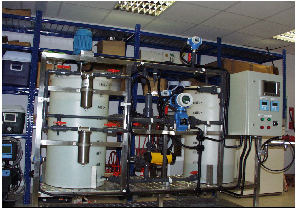
Figure 7. Lab-scale test rig for filtration performance evaluation.
